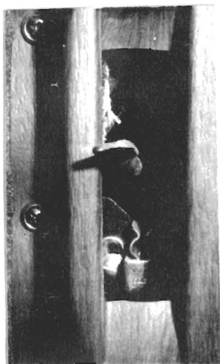
Fig. 1-7 Emergency Gear Extension Lever
